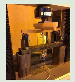
Figure 1. MOE and MOR test of TM treated lumber
